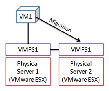
**Laserfiche Tie-in:** In the diagram above, VM1, which in this case is running a Laserfiche Server, is originally hosted on Physical Server 1. When an administrator needs to perform hardware maintenance on Physical Server 1, which will likely involve rebooting it, he/she can use vMotion to migrate VM1 to Physical Server 2. End users interacting with the Laserfiche Server hosted on VM1 will be unable to detect any difference in service—before, during, or after the migration.
