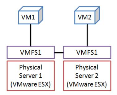
In the diagram above, VMFS1 is accessed simultaneously by Physical Server 1 and Physical Server 2.
