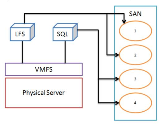
**Note:** In very high traffic situations, Microsoft SQL Server or Oracle Database can become a significant bottleneck. If you encounter this problem, we recommend having the database server run in an unvirtualized environment on a dedicated high-performance input/output (I/O) subsystem.
