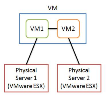
In the diagram above, there are two virtual machines (VM1 and VM2), each managed as a single unit (VM), but hosted on different physical servers (both VM1 and VM2 share the same virtual machine files). VM1 and VM2 are logically identical, representing a single virtual machine state, but they are physically distinct.
