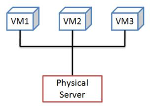
As seen in this diagram, one physical machine can host multiple virtual machines.
