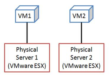
In this example, there are two physical servers. Each server is running **VMware ESXi**, which is VMware's enterprise-level hypervisor.
